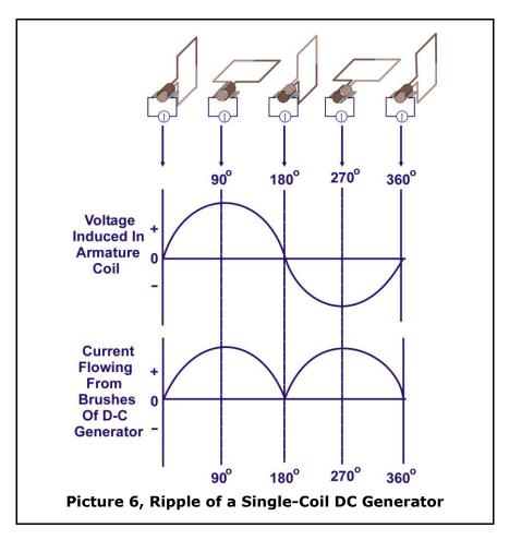
b. In practical DC generators, more coils and commutator segments are used to produce an output voltage waveform with fewer ripples. Picture 7 shows the reduction of ripple in DC voltage when two coils are used instead of one. Since there are now four commutator segments in the commutator and only two brushes, voltage cannot fall any lower than point A. Therefore, ripple is limited to voltage rise and fall between
