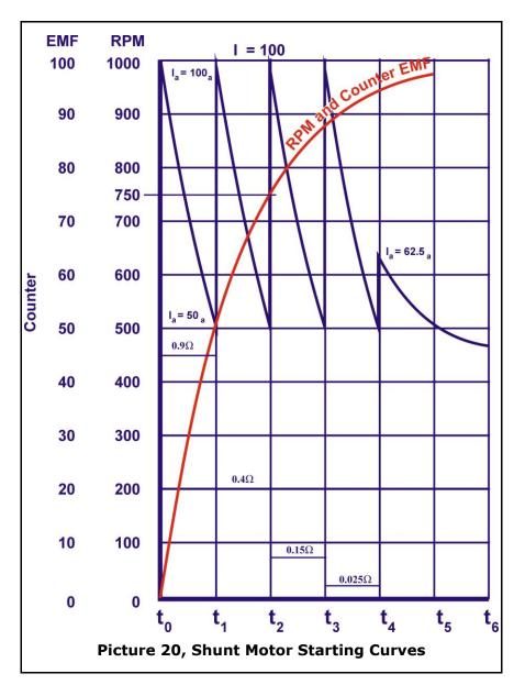
h. Initially, starting resistance of 0.9 ohms is inserted in series with the armature resistance of 0.1 ohms. Speed and counter emf voltage are zero and armature current is limited to 100 amps by the armature resistance acting in series with starting resistance.
